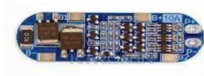
Fig 1.7 Battery Management System Module
